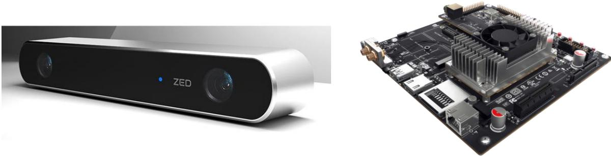
Figure 4: ZED stereo camera (left). Jetson TX development kit (right)
